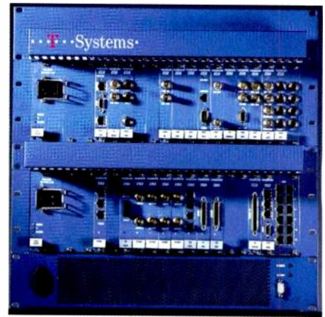
The 'Broadcast Service Multiplexer' (RfSMux) as a multifunctional network termination.
