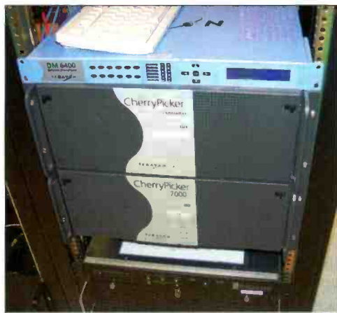
Here are two generations of cable remultiplexers. The two units on the bottom were state-of-the-art five years ago. The top unit is today's more powerful version.
