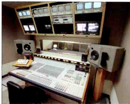
However broadcasters decide to mix, monitor and route audio, the tools they need are available. Pictured: A Wheatstone TV-80 at WGCL-TV in Atlanta. Photo courtesy DST.
