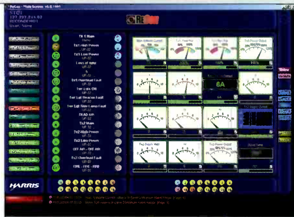
Figure 1. This remote control system base screen provides access to control (left side), monitoring (center) and metering (right side) functionality. Base Recon screen courtesy Harris.
