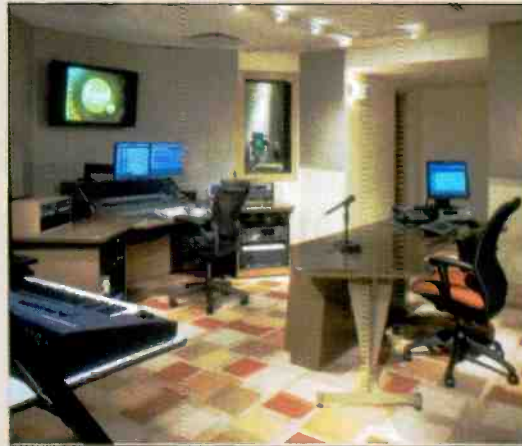
A Solid State Logic C100 console, a portable Yamaha mixing board, and other tape decks and audio peripherals in the audio control room provide a generous helping of digital audio for facility productions. Access to a voice-over booth in the post digital audio room is also available.
