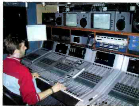
PrimeVision uses the Studer Vista 8 console to record live audio in its HD30 remote truck.
