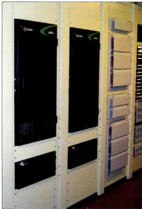
NVISION's NV8256-Plus router features a high-density 256x256 crosspoint module. Its frame has provisions for an additional crosspoint module to serve as a hot standby, eliminating the crosspoint module as a single point of failure in the system.
