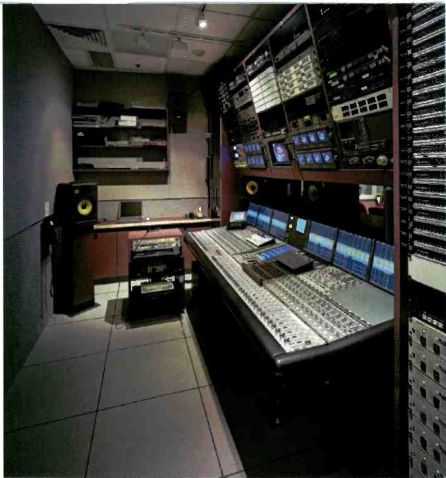
An SSL C100 digital broadcast console generates 5.1 surround, stereo and mono mixes for production and distribution to Comcast SportsNet's two stadium locations: the Wachovia Center basketball/hockey arena and Citizens Bank Park baseball stadium.
