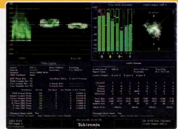
▲ Displays of video and audio with sessions screen provide quick signal monitoring of the signal.
