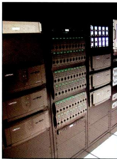
WJLA-TV uses 26 channels of DV25 for news editing and more than 16 channels of MPEG-2 for playout. Shown is a Leitch SAN architecture storage system.
