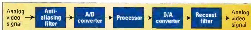
Figure 1. Block diagram of a typical black box digital device. It can represent any digital device in use in a teleproduction facility.
