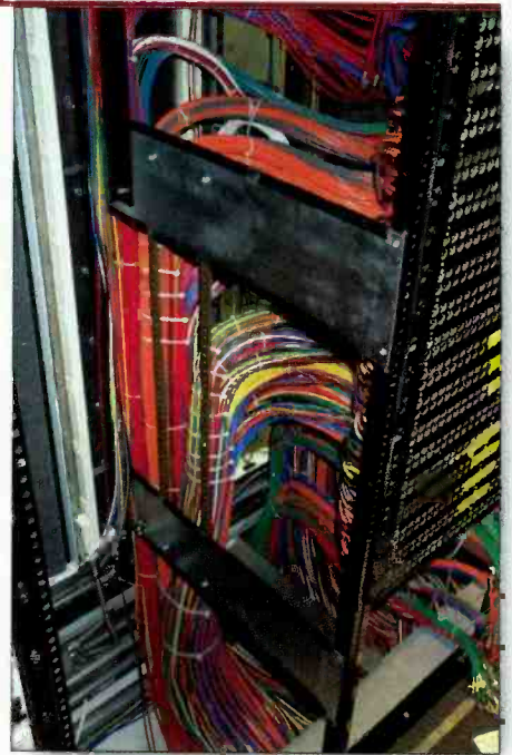
Careful cable choice and neat installation can help alleviate airflow and weight issues in truck construction.
