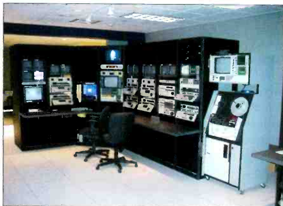
FSNNE's videotape location contains six Sony SX decks, three Sony Beta decks and a single ¾-inch deck with some dubbing capacity.
