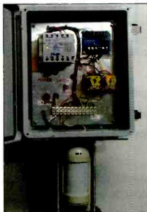
The Resonant Results' Tower Watcher TW-100 model has power supply, remote control interface, and a sensor as one unit. It separates the electronics and the detector outdoors and the electronics indoors.
