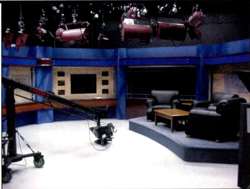
Camera work at the FSNNE studio is handled by two Sony handheld cameras, one of which is on a jib, as well as two Sony studio cameras.
