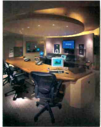
In WNET's New York audio production suite, columns and a need for corner seating required the creation of an asymmetrical version of a railroad room layout.
