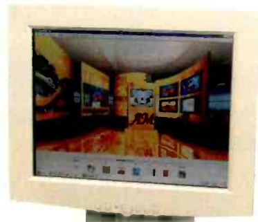
Users interact with the virtual set through an intuitive touch-screen interface that shows the entire set from the director's chosen viewpoint.
