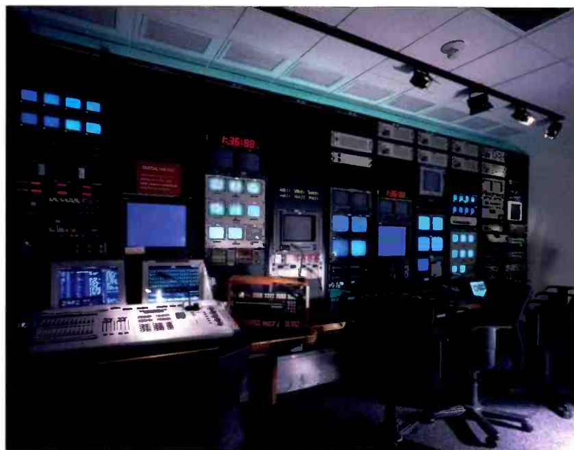
Production at CNN's new facility takes place not only in the studios, but also in technical spaces like the lighting and video shading room shown above.
