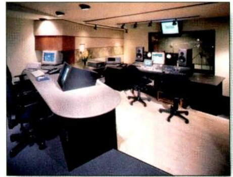
New York audio post house Superdupe features a railroad-layout room design, with partially asymmetrical furniture arrangement, but symmetrical room boundaries and acoustic surfaces.
