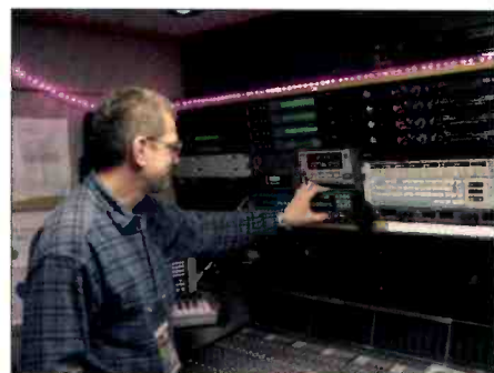
NMT's DX11 was linked with two other trucks covering the Super Bowl via a 384-port system created by linking Telex ADAM intercom systems.
