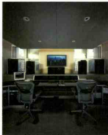
Carter Burwell's private production studio is a symmetrical arrangement of the cockpit style. In a cockpit-style room, the console or workstation is located on the room's physical centerline, with all other equipment arranged as symmetrically as possible around it.
