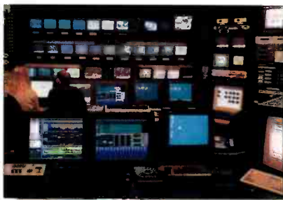
Production-control-room automation systems like ParkerVision's can replace a room full of hardware and reduce staff.
