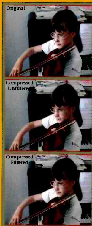
Figure 1. MPEG-4 part 10, or Advanced Video Coding, uses reconstruction filtering to minimize the perception of the blocking artifacts common with earlier MPEG standards. The image sequence above includes the original, the result after AVC encoding/decoding, and the final result after reconstruction filtering. Images courtesy of Iain Richardson.
