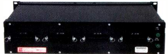
PPA3-14MKIIANS 2 RU Longframe Evenly-Spaced 2x24 AMP 50-Pin Receptacle Patchbay (Rear View)
