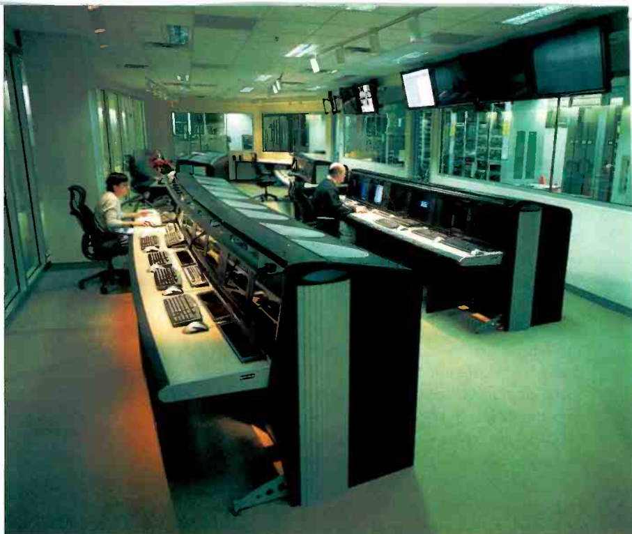
The media operations control center is the broadcast equivalent of an air traffic control center for the coordination of playlist changes and ingest operations.
