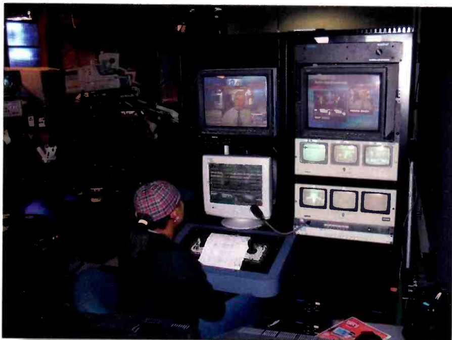
The control positions were located within the two studios to provide a more intuitive feel for the operator.
