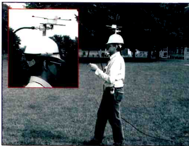
Evaluation of proposed ATSC enhancements to the 8-VSB modulation system have included testing of "walkabout portability" using the test configuration pictured in the images above; the separate receiver is not shown. Note the wireless phone and headset used for communications between test personnel.
