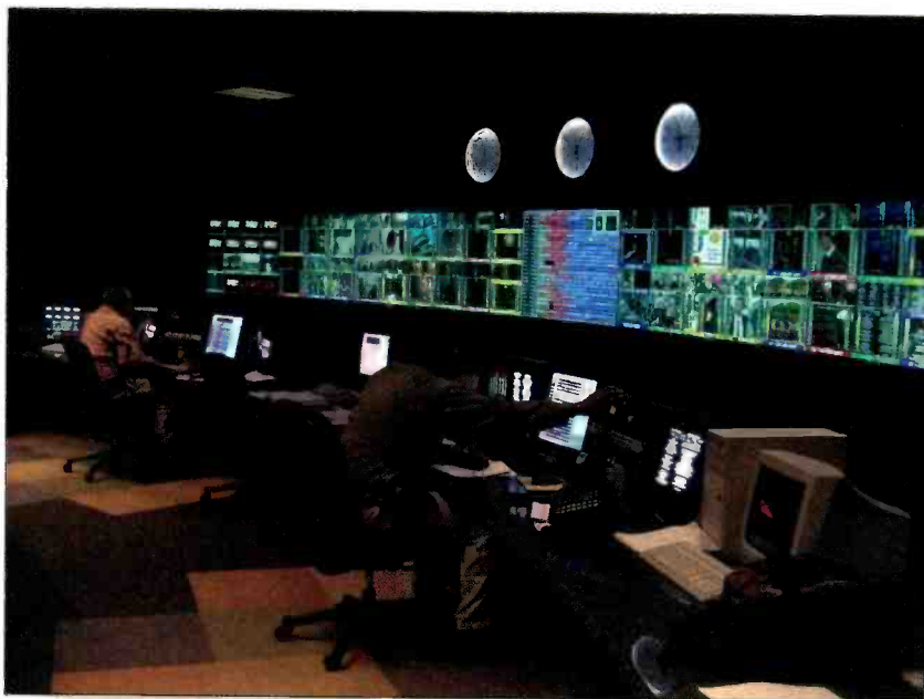
Operators at Starz Encore's broadcast operations center monitor 26 primary channels and 26 backup channels using the Omnibus Colossus automation system.
