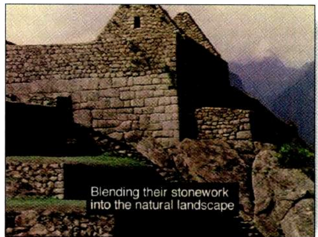
Figure 1. Sample of 708-style closed captioning. Note the variable transparency of the text block. Courtesy of WGBH.
