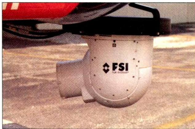
The Ultramedia III camera from Flir Systems is equipped with a Sony BVP-570 camera and a Canon 1000mm lens, all contained in the "ball" located underneath the WPIX-TV helicopter.
