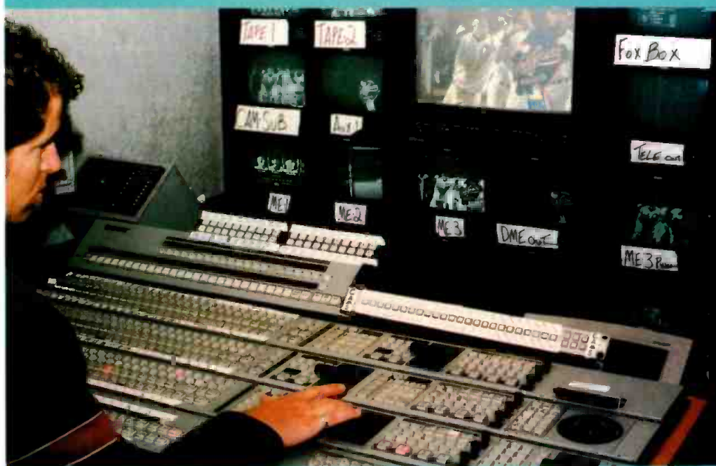
Sony DVS-7350/DME7000 production switcher used in coverage of the Fox Networks 2000 World Series broadcast. Photo by Ben Luzon.
