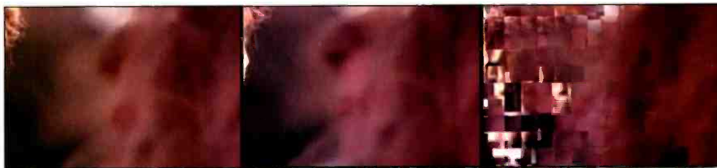
Figure 2. Lost packet in an I frame results in severe blockiness in a neighboring B frame.
