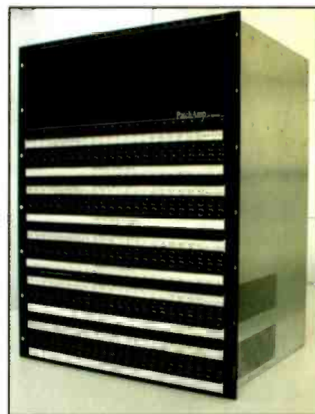
The PatchAmp patching and distribution system enables broadcasters to eliminate unnecessary wiring using five 24-position patch panels and 24 1x5-distribution amplifiers. Sources within the system are oriented horizontally and destinations are arranged vertically.
