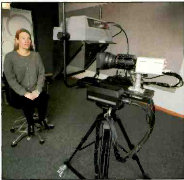
The studio's Sony DXC-950 camera with ESI robotics (shown above) was positioned by an operator in communication with broadcasters via a coordination phone line.
