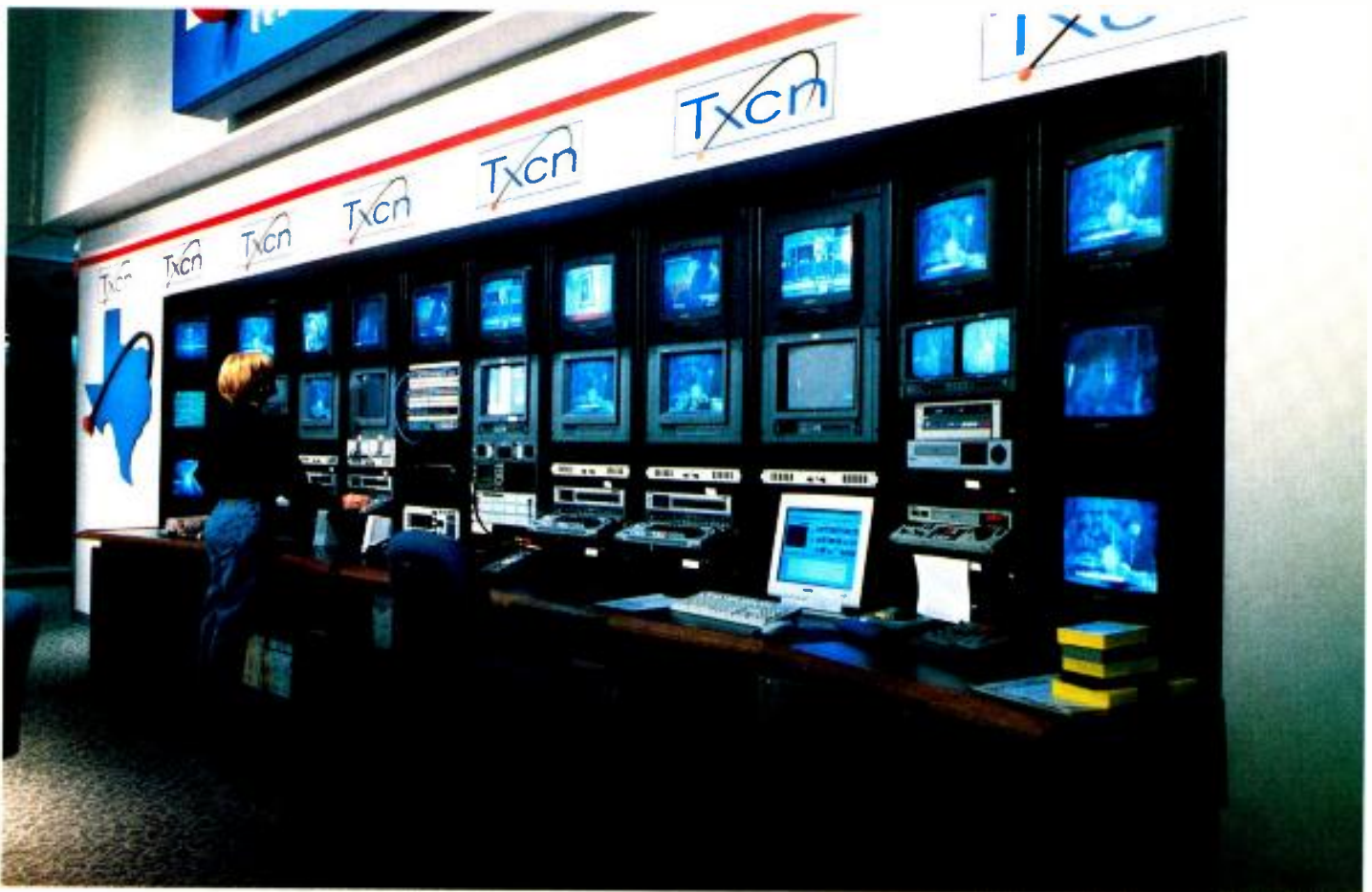
Nonlinear editing capabilities at Texas Cable News, Dallas, include Sony DNE-1000 editors networked to a central server system. This kind of arrangement allows non-technical staff to edit the news content they are producing. Photo courtesy Concept: Benson & Rice.
