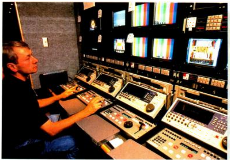
Panasonic's HD truck, which also saw use during a full season of Monday Night Football broadcasts, features a complement of Panasonic AJ-HD2700 HD-D-5 multiformat VTRs.
