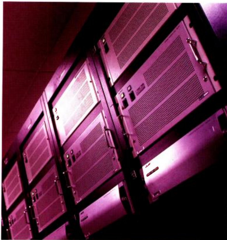
Servers, such as these Sony MAV-70s, use varying levels of MPEG compression, reducing the need for expansive tape libraries. Keeping large archives available electronically allows content can be recalled to individual workstations for use by working journalists and editors. Photo courtesy Concept: Benson & Rice.
