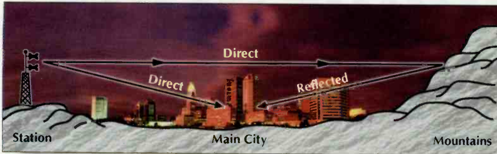
Multipath results from a single point receiving the same signal from two or more sources. The direct signal is usually the strongest.
