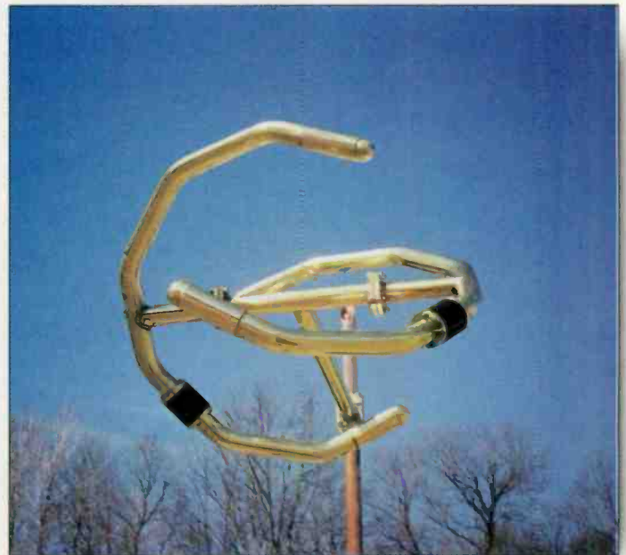
A higher frequency means a smaller wavelength. Because of this, an FM antenna can be only a few feet long instead of several hundred feet, like an AM radiator. (Photo courtesy of Propagation Systems Inc.)
