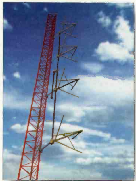
By adding additional radiating elements, the radiated beam is narrowed and provides increased power gain. (Photo courtesy of Antenna Concepts.)
