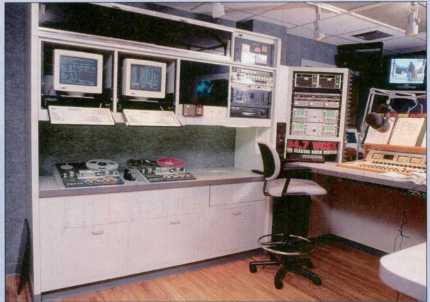
The on-air control room at WCSX, Detroit, uses PCs for data management and a Radio Systems DDS for audio delivery.
