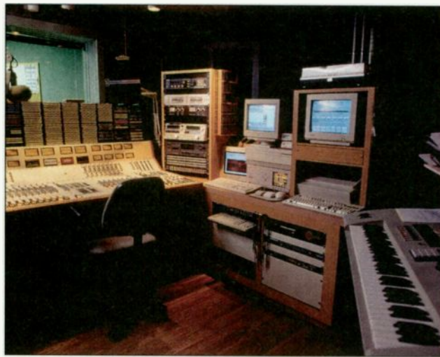
Production Studio No. 1 at WCSX, Detroit, shows the growing influence of computers in radio. It includes a digital audio workstation, a control terminal for the station's on-air delivery system, a digital audio sampler/synthesizer and ISDN-connected receivers for two file-based audio transmission networks.
