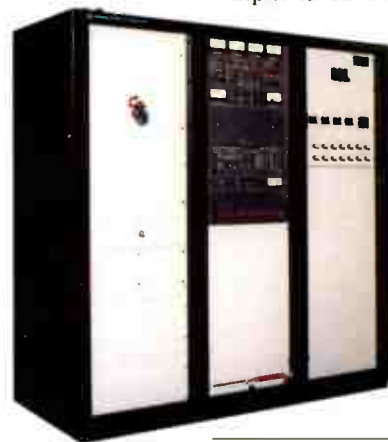
The Continental 816R series is an example of hybrid FM transmitter design. It combines a solid-state exciter and an IPA with a tube final stage for powers ranging from 21.5kW to 35kW.
