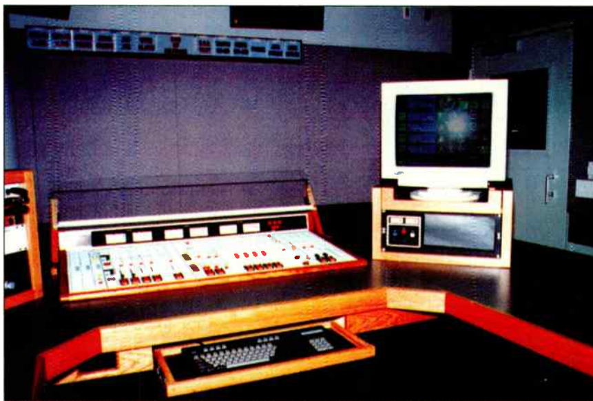
Many of today's studios control audio signals with a "hybrid" approach, combining conventional mixers with computer-based storage.
