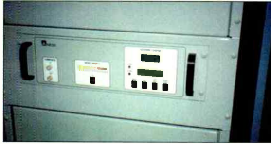
Digital FM exciters like the Nautel NE-50 are typically available with either analog or AES/EBU digital audio inputs.
