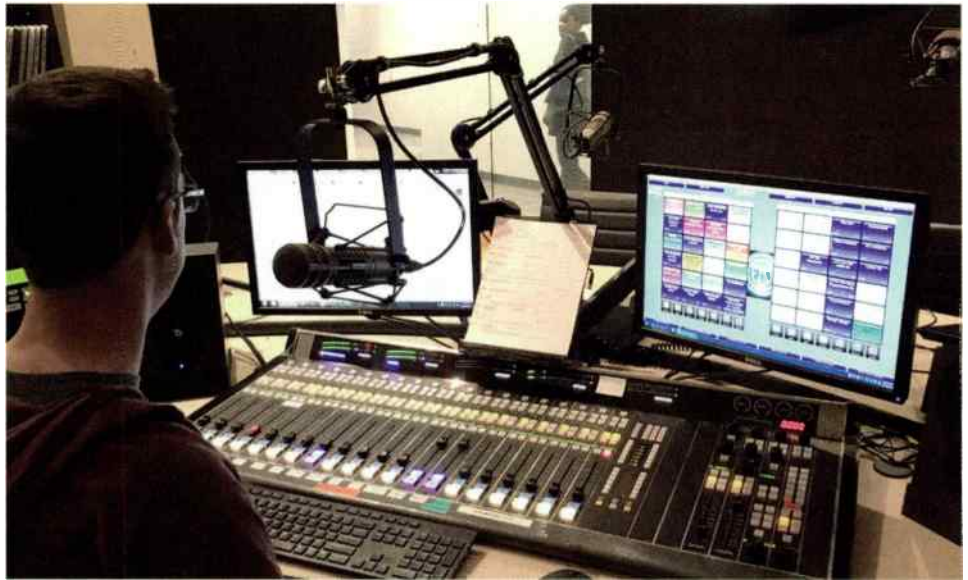
WFPK Studio 1 with Wheatstone LX-24 and VX drop-in and ENCO DAD.
