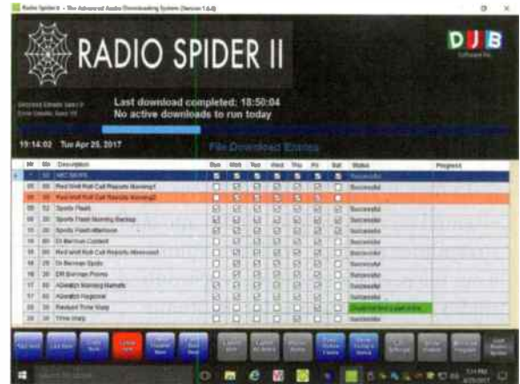
Fig. 1: Radio Spider is used to automatically download news, spots and shows from FTP and HTTP sites, as well as from folders that contain individual show downloads.
