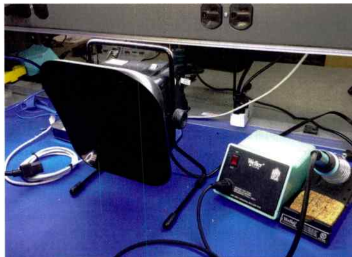
The solder fume extractor should naturally be placed adjacent to your soldering station.
