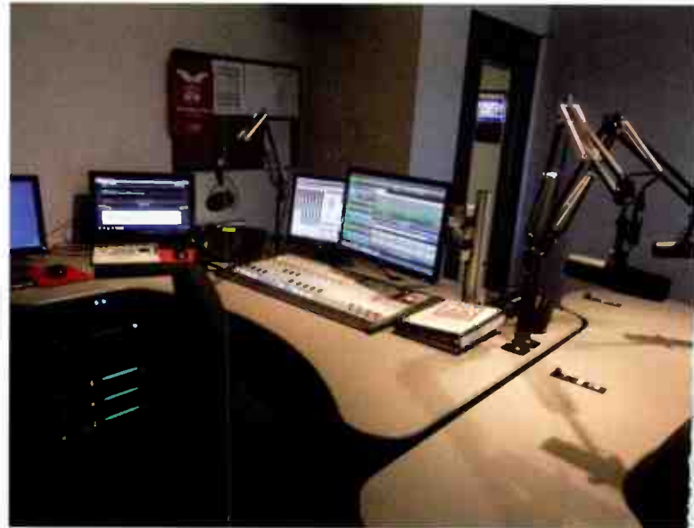
The Bob 107.9 studio has a slightly different configuration because of the room dimensions. The guest area is to the side instead of to the front of the console.
