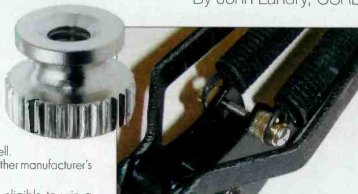
A thumb nut and screw installed on a mic boom. Thumb nuts (inset) are available at most hardware stores.
