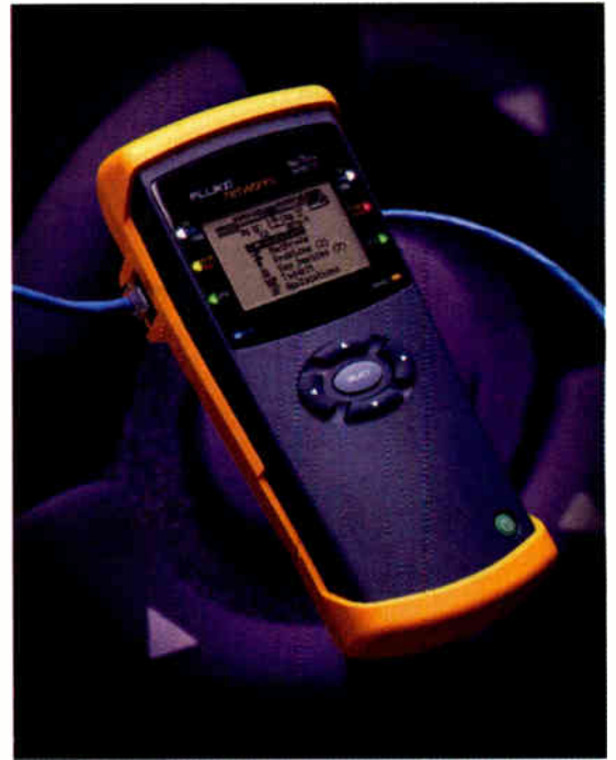
Ethernet testers, such as the the Net Tool Series II from Fluke, are the modern handheld test tool in an IT-based facility.
