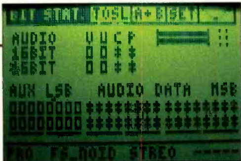
Figure 3. The display showing a bit-depth of 16 bits. For a 24-bit signal, the left-most (LSB) boxes would not be empty.
