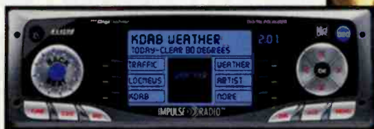
Providing data in addition to the audio is a subcarrier function that is being carried over to DAB.
