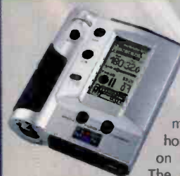
The Mayah Flashman records onto Compact Flash cards, which allow more than eight hours of recording on a 256MB card.
