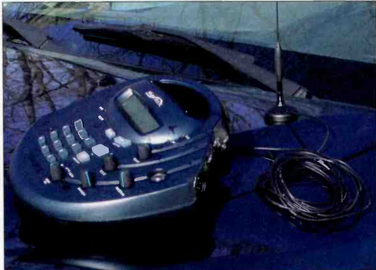
Comrex has introduced a GSM wireless module that simplifies accessing the wireless network with a codec.
