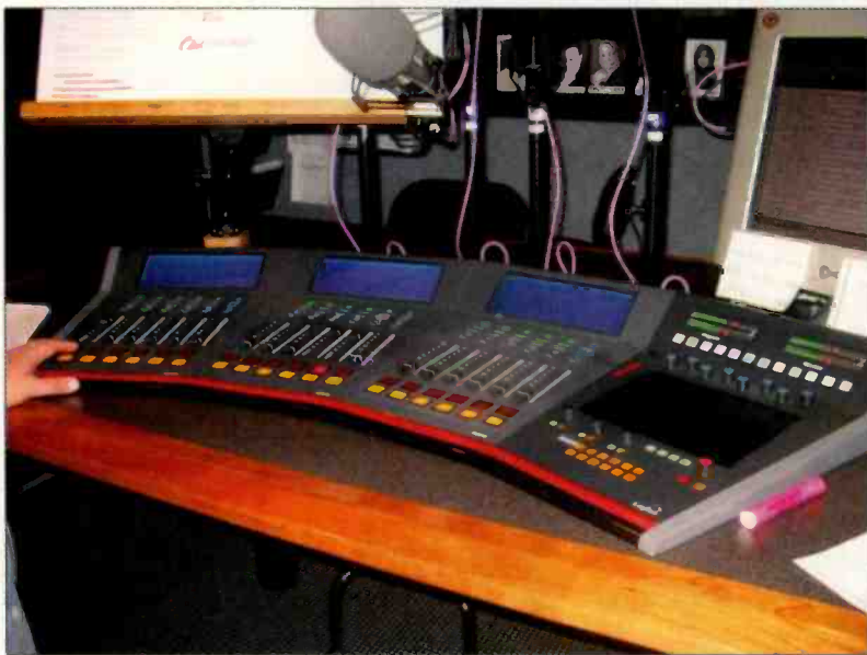
Through a greater degree of integration, the console surface can display more information to the operator.
