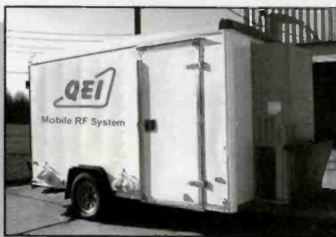
Transportable Pre-Built Transmitter Sites
