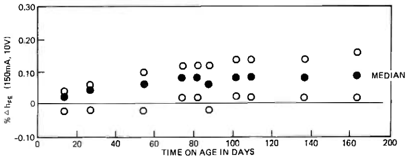
Fig. 7—Stability of a group of transistors during long-term aging.
