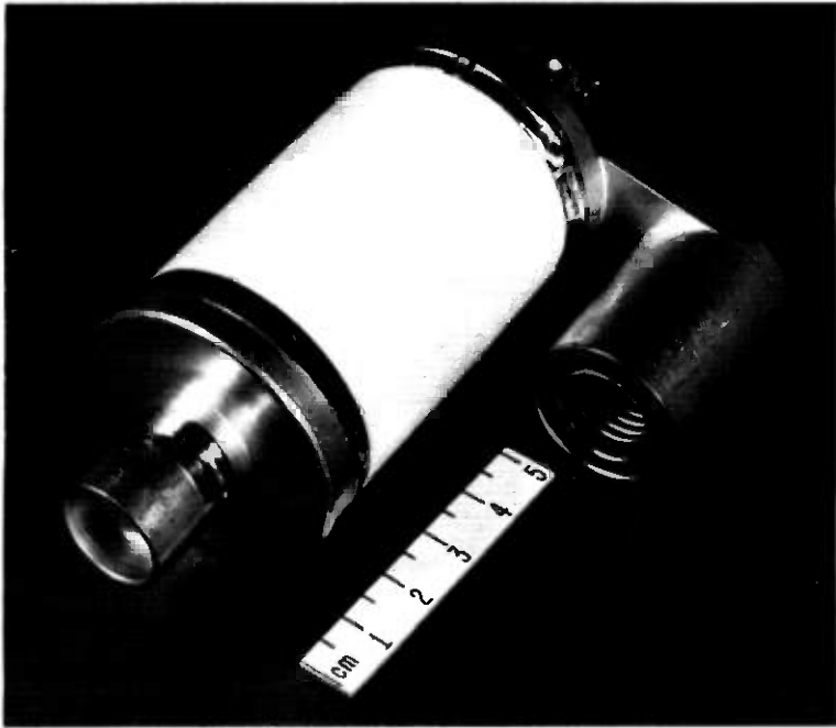
Fig. 12—Completed coaxial capacitor used in ground separation filter. Note expansion bellows.
