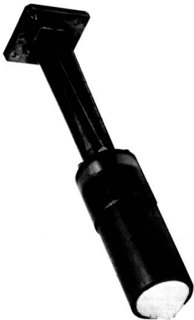
Fig. 9—Dual mode feed: (a) photograph showing insect seal; (b) diagrammatic depiction of seal.
