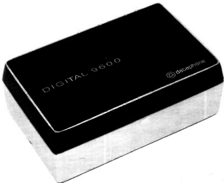
Fig. 9—Channel service unit.
