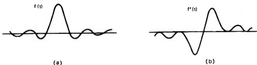
Fig. 1—(a) Original pulse. (b) Phase-distorted pulse.
