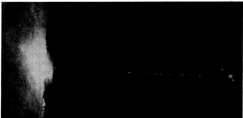
Fig. 4—Propagation of light beam guided in a strip-loaded guide. At the point where the strip is scratched, the light is radiated.
