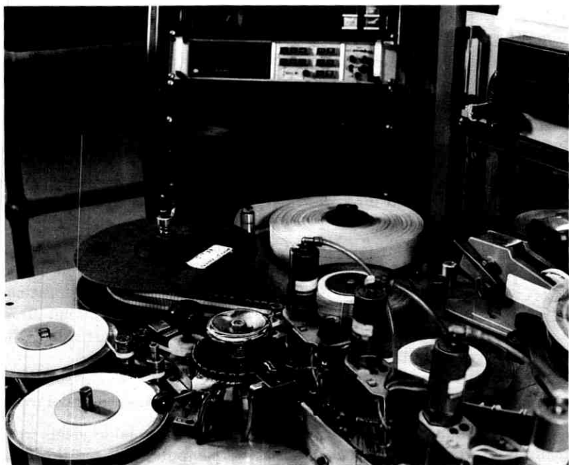
Fig. 6—Resistor taping station on radial sequencer machine with test station in background.
