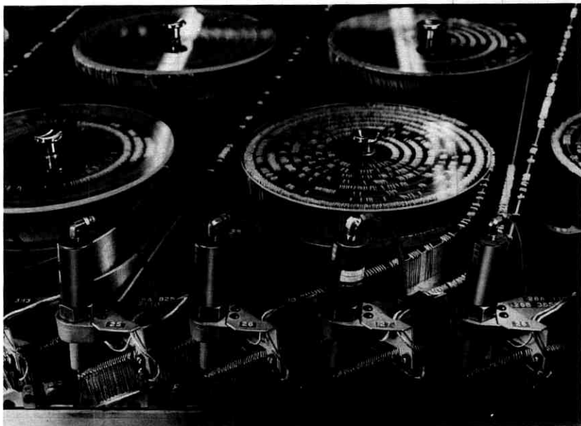
Fig. 5—Resistor containers on radial sequencer machine.
