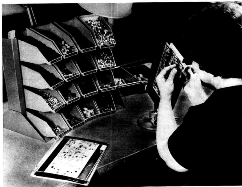
Fig. 1—Hand insertion position showing components in the rack and the board holder with PWB.
