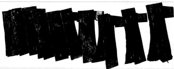
Fig. 13—Specimens of the five rubber-to-aluminum bonded combinations retrieved from two depths after four years soil burial exposure at Roswell. All bonds have failed due to severe corrosion.
