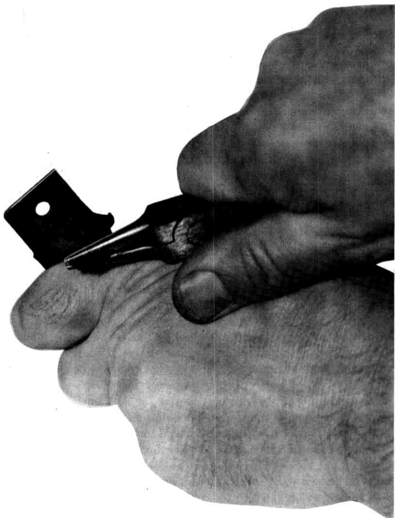
Fig. 11—Hand-peel test used to determine the strength of rubber-to-metal bond. Specimen is #275-SBR compound M-206 bonded to stainless steel with the Chemlok 201 plus Chemlok 220 system—after retrieval from Bainbridge.
