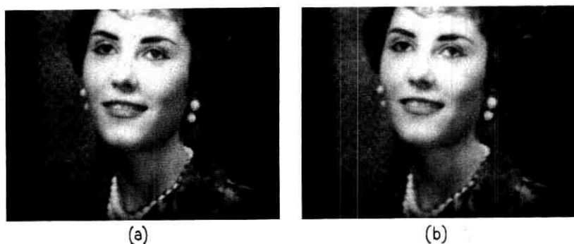
Fig. 8—(a) Analog Picturephone signal "Rosalie." (b) Photograph of 3-bit DPCM encoded Picturephone signal "Rosalie." Exhibit of slope overload.
