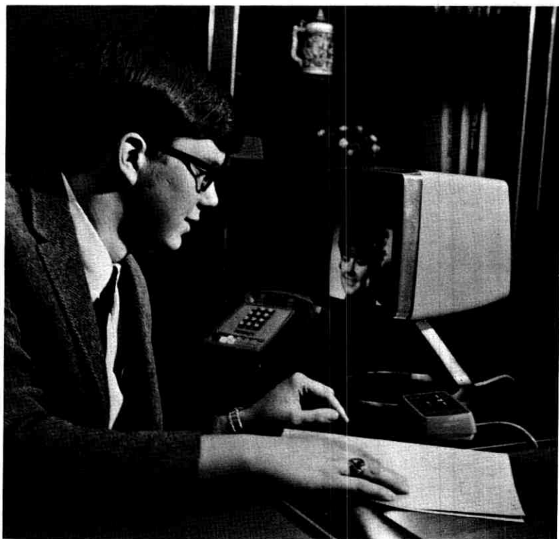
Fig. 1—The station installation, showing three of the four components: the existing telephone, a display unit, and a control pad. (The service unit is not shown.)
