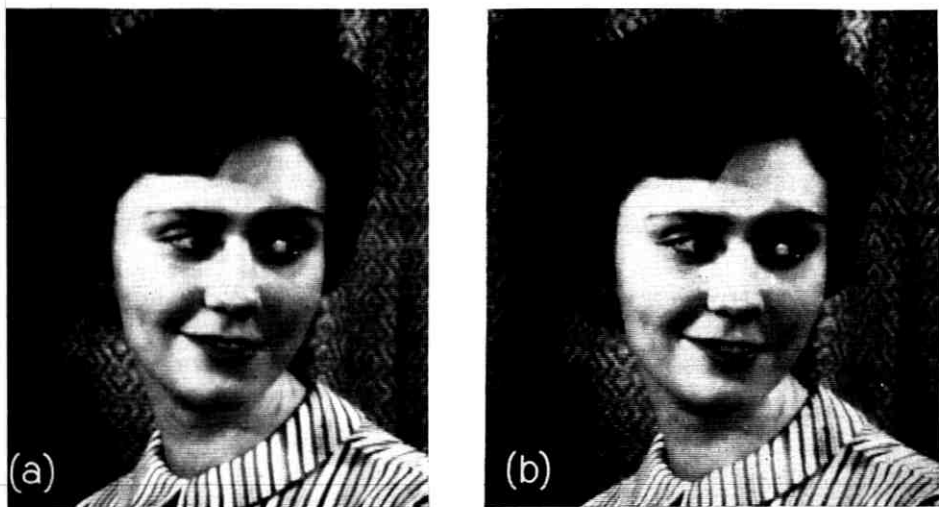
Fig. 10—Results of a video simulation: (a) 20 MBPS PCM original (b) 10 MBPS ADM output.
