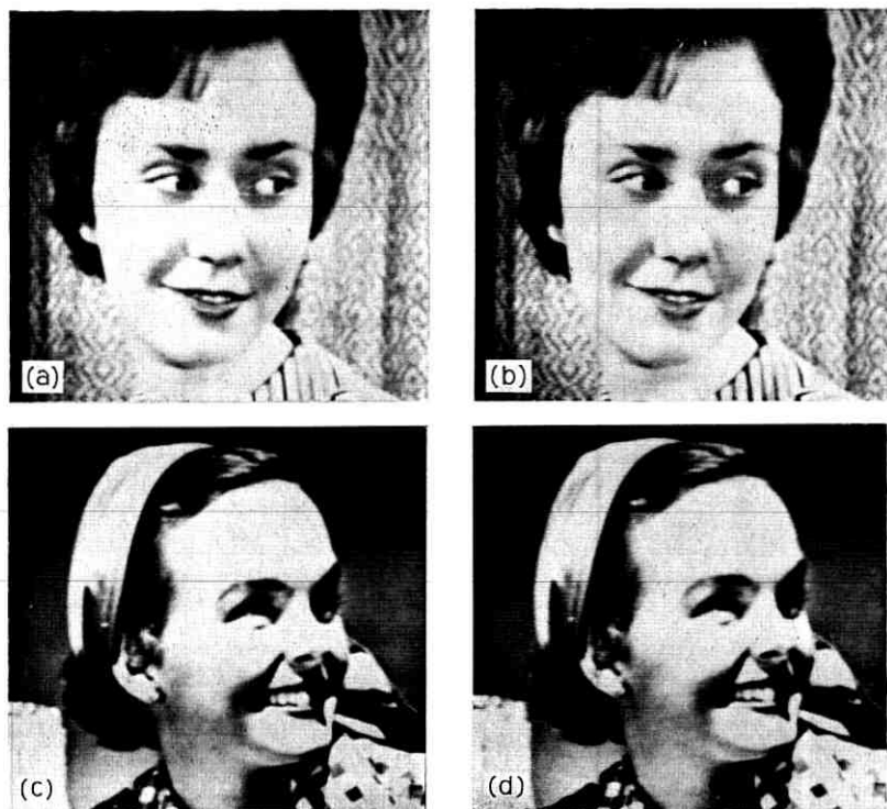
Fig. 8—Photographs of television pictures bandlimited to 1.0 MHz: (a) high detail picture without coding, (b) high detail coded picture with optimum input signal level, (c) low detail picture without coding, and (d) low detail coded picture with optimum input signal level. (The scan lines and printing screen in Figs. 8 through 11 cause moiré patterns that are not in the originals.)
