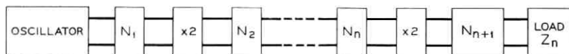
Fig. 7—Lossless abrupt-junction varactor multiplier of order 2^n . Only AM (or PM) ports of the doubler and interstage networks are shown in the figure.
