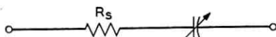
Fig. 1—Varactor model consisting of a constant resistance in series with a time-varying capacitance.
