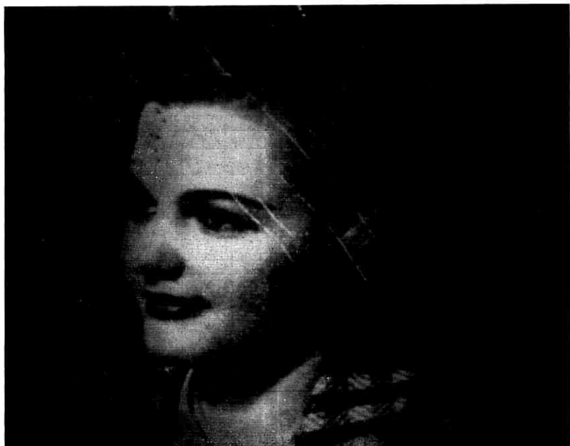
Fig. 2—Photograph obtained with the 540 \times 540 diode array target. The subject was a black and white transparency illuminated with a tungsten lamp.
