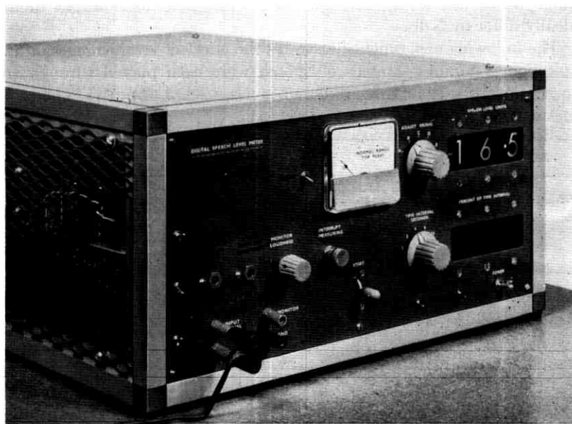
Fig. 12—Digital speech level meter.
