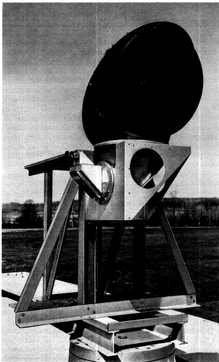
Fig. 5 — The antenna model mounted for radiation pattern measurements in the transverse plane and 0^\circ elevation.
