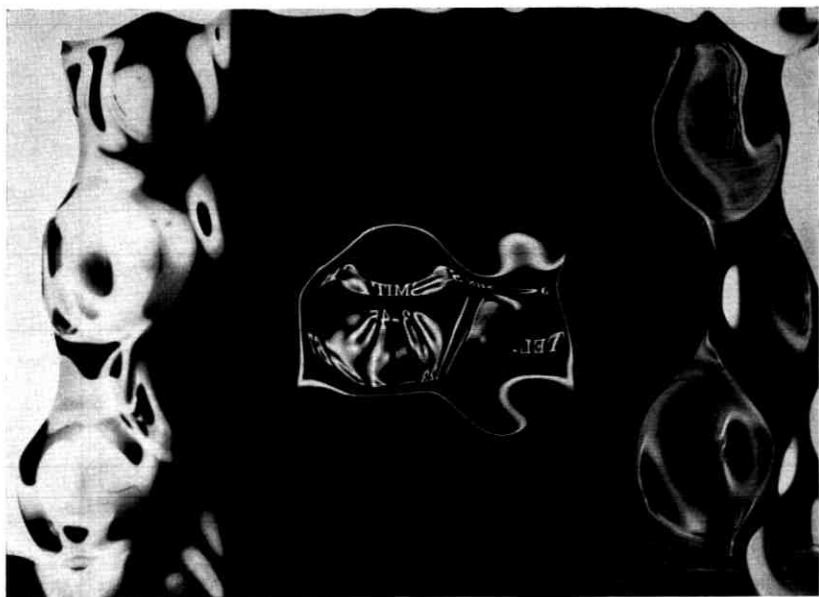
Fig. 2—Object text photographed through warped glass plate.
