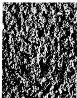
(a) SURFACE NO. 1 BLASTED WITH NO. 60 QUARTZ GRIT AND ELECTROPOLISHED MAGNIFICATION 42X
