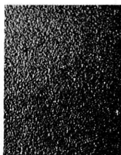
(c) SURFACE NO. 3 BLASTED WITH STAINLESS STEEL BALLS AND ELECTROPOLISHED MAGNIFICATION 42X
