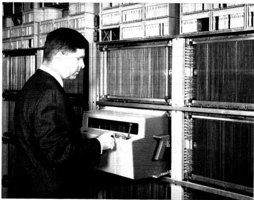
Fig. 29 — Card loader in use on program store.
