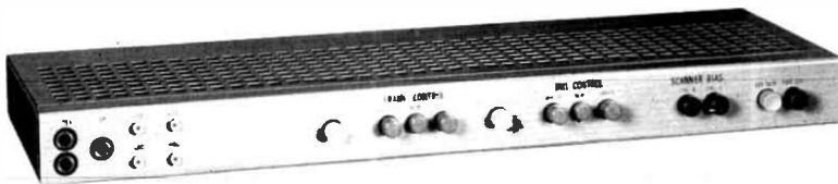
Fig. 3 — Typical frame control panel.
