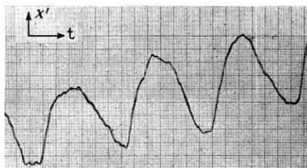
Fig. 17 — \chi' signal for rapid adiabatic passage, when T_1 is not very small compared with the field modulation cycle. Compare with Fig. 14(c). No phase sensitive detector is used here (therefore, considerable drift is observed).
