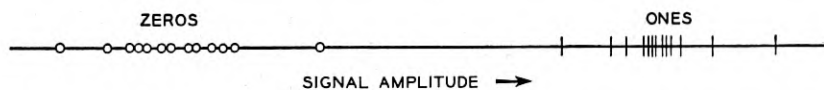
Fig. 12 — A possible set of signals from each site in a binary store, showing a range of signal variations.
