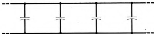
Fig. 6 — Capacitances connected across a smooth transmission line periodically couple the forward and backward waves and produce stop bands characterized by growing and decaying waves.
