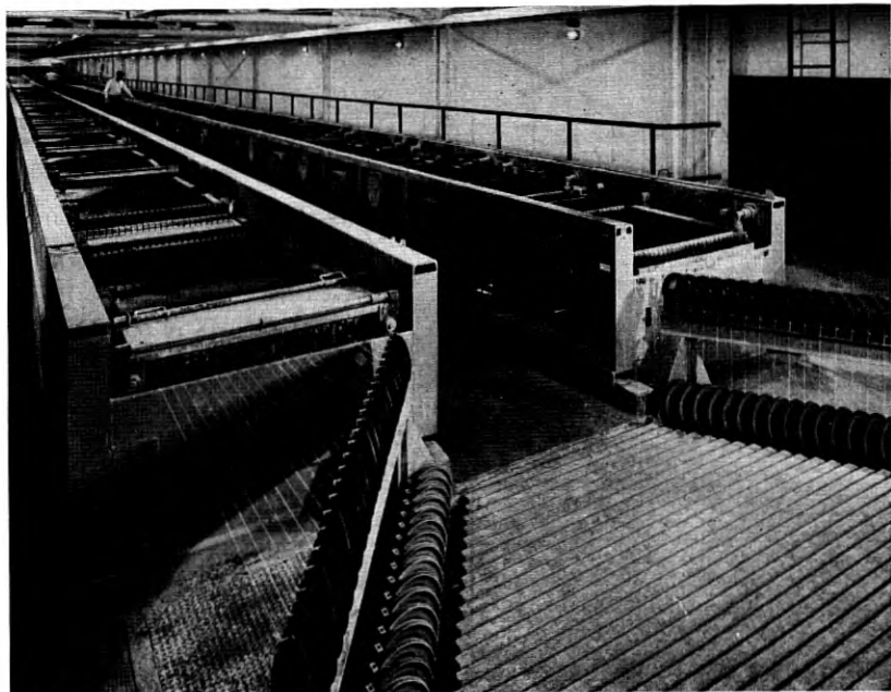
Fig. 6 — Turning section of the machine where the twenty-five channels of wire, after having been cleaned and partially plated in the tanks on the left, reverse their direction and travel the full length of the building, receiving added copper coating in the series of plating cells.
