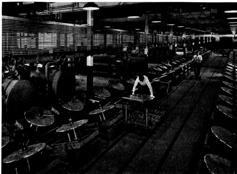
Fig. 1 — Steel wire supply stands, two for each of the twenty-five channels on a machine, permit continuous operation. A 450-lb. spool of wire is being positioned by the nearest operator while behind him another operator is electric welding a wire joint.
