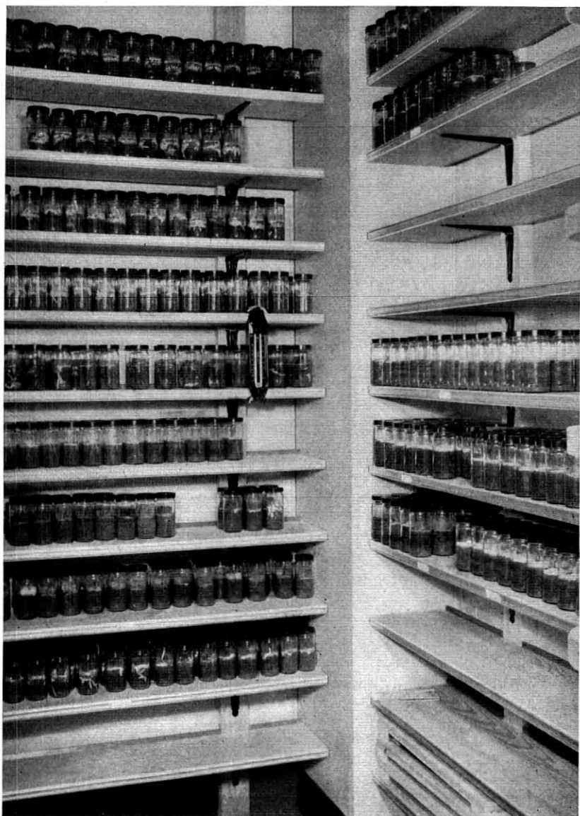
Fig. 2—Soil-block cultures on the shelves in the incubation room. The unpainted wood shelves come to equilibrium with the temperature and relative humidity and thus are a factor in keeping the conditions stable. The back edges of the shelves are set away from the wall to provide spaces for air circulation. The front edges of the shelves are provided with metal labeling strips.
