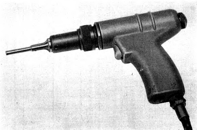
Fig. 37—Wrapping tool operated by air pressure for factory use.
