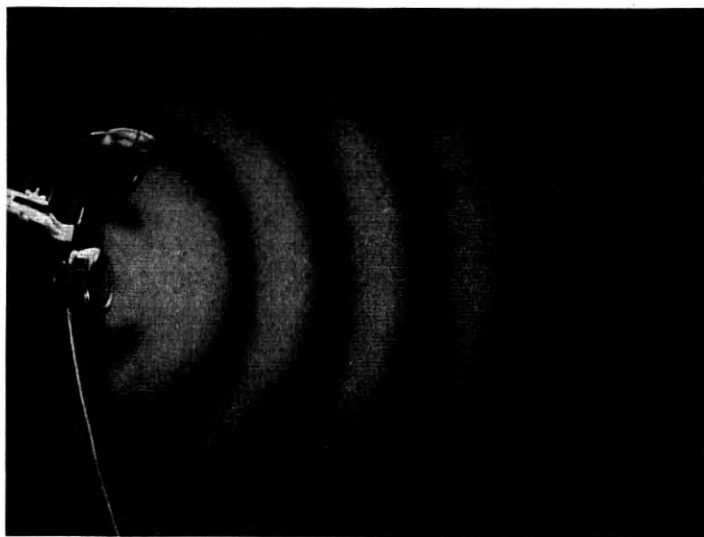
Fig. 30—A pattern of a carbon telephone transmitter obtained by the transposition method of Fig. 29. The phase fronts are those which would be observed if the microphone were radiating sound. f = 4 KC ( \lambda = 3.4'' ).
