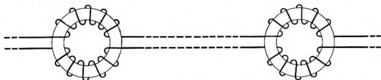
Fig. 1—Non-phantom type loading coils. Coil winding schematic and method of connection into circuit.
