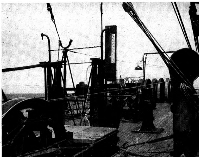
Fig. 14—Ring sheave and dynamometer scale.
