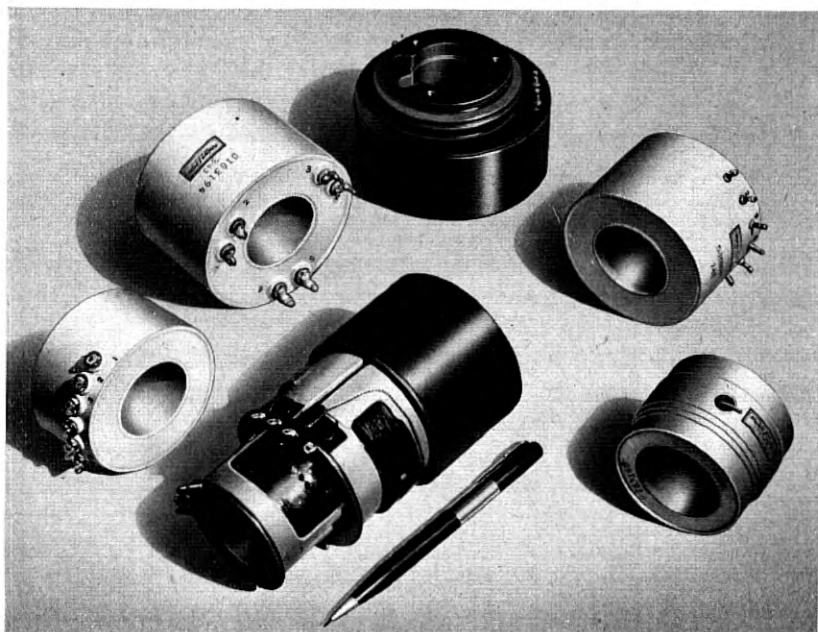
Fig. 40.—Typical magnetic focus and deflection coil designs as developed for military radar purposes.
