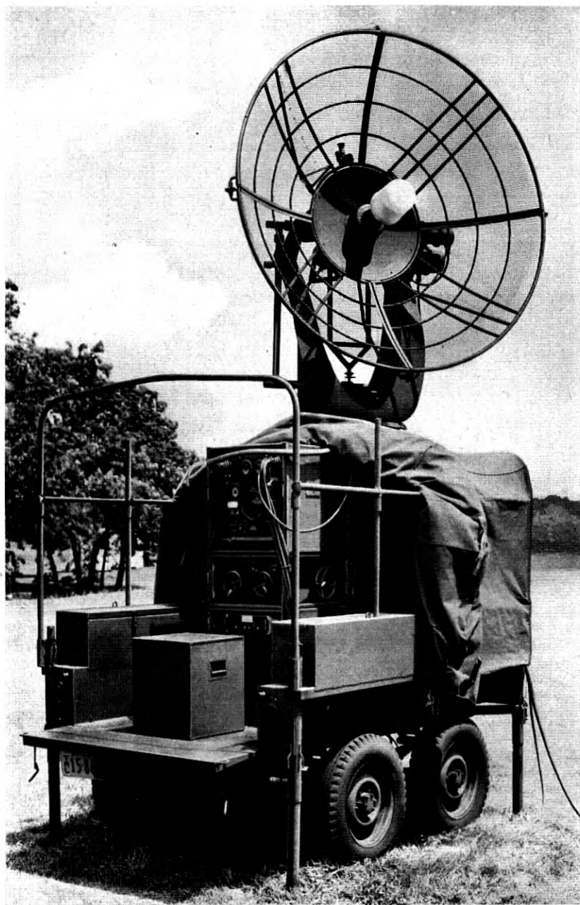
Fig. 1.—Radar Equipment—Mark 20. This mobile equipment operating at 1000 mc is employed for searchlight control purposes.
