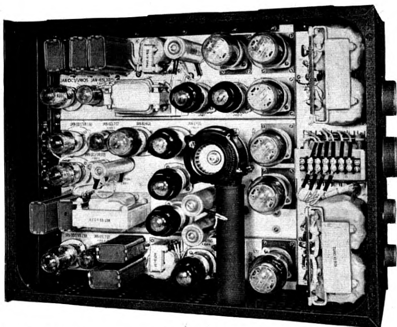
Fig. 73.—Low-voltage power supply for AN/APQ-7 airborne radar system—Mechanical features.
